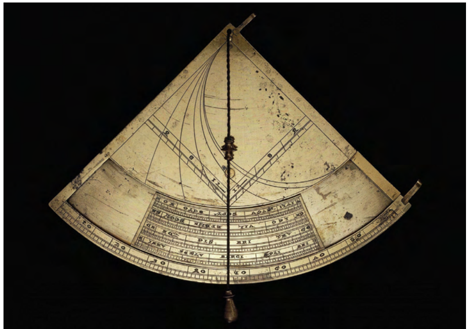
Above: The British Museum quadrans vetus , an unequal-hour quadrant with moving cursor. © Trustees of the British Museum.
